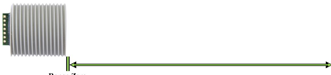
**The range is measured from the front of the transducer to the target.**
