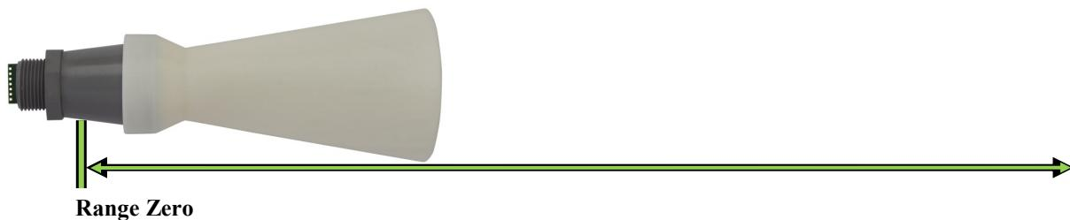
The range is measured from the front of the transducer to the target.
