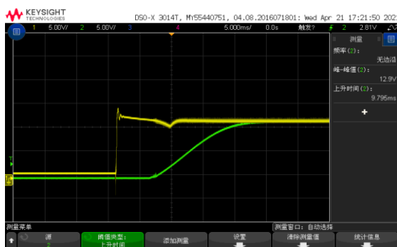
Figure 6, Output voltage established (Iout = 6A)
