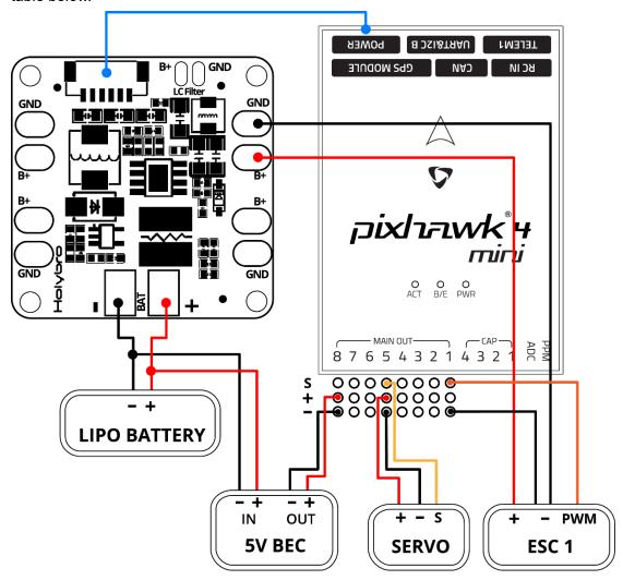
Note: The image above only shows the connection of a single ESC and a single servo. Connect the remaining ESCs and servos similarly. Refer to Airframe Reference (https://docs.px4.io/en/airframes/airframe\_reference.html) to connect ESCs to **MAIN OUT** in the correct order for your airframe configuration.
