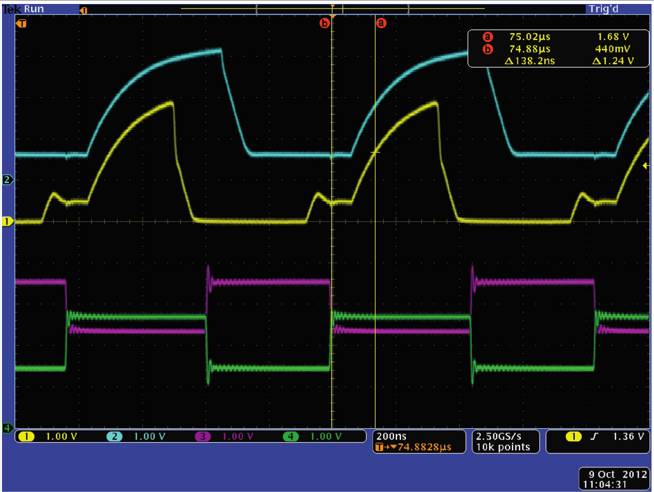
Figure 11. Differential bus waveform
