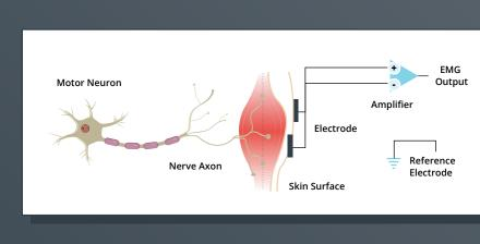
The difference in voltage between the two electrodes is amplified with respect to the reference electrode. The advantage of this configuration is the common noise between the two electrodes is removed due to the amplifier's common mode rejection ratio (CMRR).
