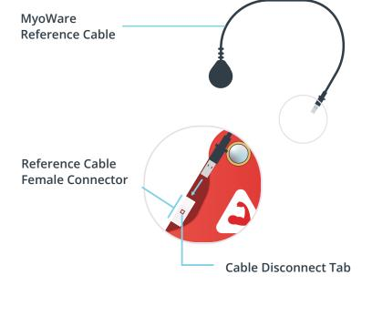
Insert the MyoWare Reference Cable into the female connector located on the left side of the sensor. Remove the cable by pressing
