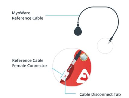
Insert the MyoWare Reference Cable into the female connector located on the left side of the sensor.
