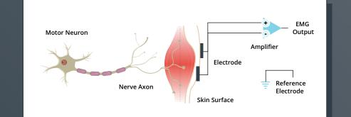
The difference in voltage between the two electrodes is amplified with respect to the reference electrode. The advantage of this configuration is the common noise between the two electrodes is removed
