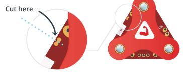
Reference Electrode Socket Disconnect Jumper
