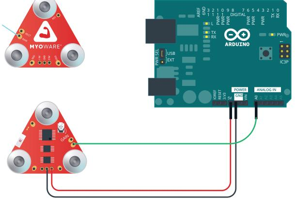
To output the raw EMG signal, simply connect the RAW pin to your measuring device instead of the ENV pin.
