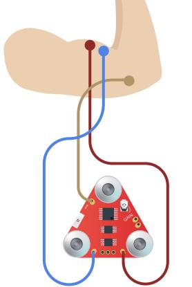
electrode placed adjacent to the middle electrode towards the end of the muscle body
