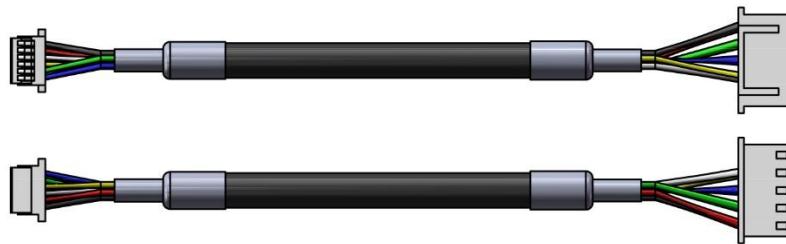
Figure 2-6 RPLIDAR S1 Interface Lead Schematic Diagram
