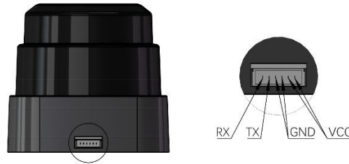
Figure 2-5 RPLIDAR S1 Female Receptacle Definition
