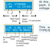
At this screen, you can set up the current and voltage of the battery pack. Charging and discharging will make the batteries come to the voltage level of "storage" state.
