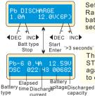
Set up the charge current on the left and nominal voltage on the right. Range of discharge current is 0.1-5.0A, the voltage should match the battery being charged. Press START/ENTER key for more than 3 seconds to startcharging.
