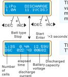
The value of discharge current on the left can not exceed 1C, and the value on the right can not be under the voltage recommended by the manufacturer to avoid deep discharging. Press START/ENTER for more than 3 seconds to startcharging.
