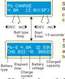
Set up the charge current on the left and nominal voltage on the right. Range of current is 0.1-5.0A, the voltage should match the battery being charged. Press START/ENTER key for more than 3 seconds to start charging.
