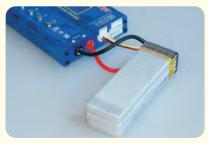
The main battery leads must be connected along with the balance lead connector as shown before charging your battery ..
