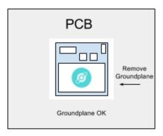
In all cases, the requirement to run traces under the module may arise. This is allowed provided there are no traces run through the RF KEEPOUT area described in the Recommended Pad Layout section above. Beware that high speed data lines running under the module is not recommended as there might be interference in both directions (host to module and module to host) especially when the module executes a transmission.
