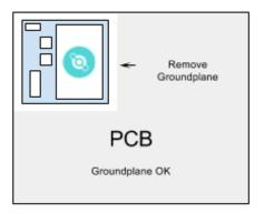
Based on the above recommendations, there may be situations where you cannot place the module near an edge. This may force the module to buried within the center groundplane of the host base board. Even though this is not recommended due to the dramatic decrease in chip antenna performance, the U.FL connections will still provide adequate RF performance to the external antenna of choice. As long as the ground plane can be minimized under the module as shown in the following figure.
