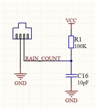
The rain gauge is a self-emptying tipping bucket type. Each 0.2794mm of rain cause one momentary contact closure that can be recorded with a digital counter or microcontroller interrupt input. The gauge's switch is connected to the two center conductors of the attached RJ 11-terminated cable.
