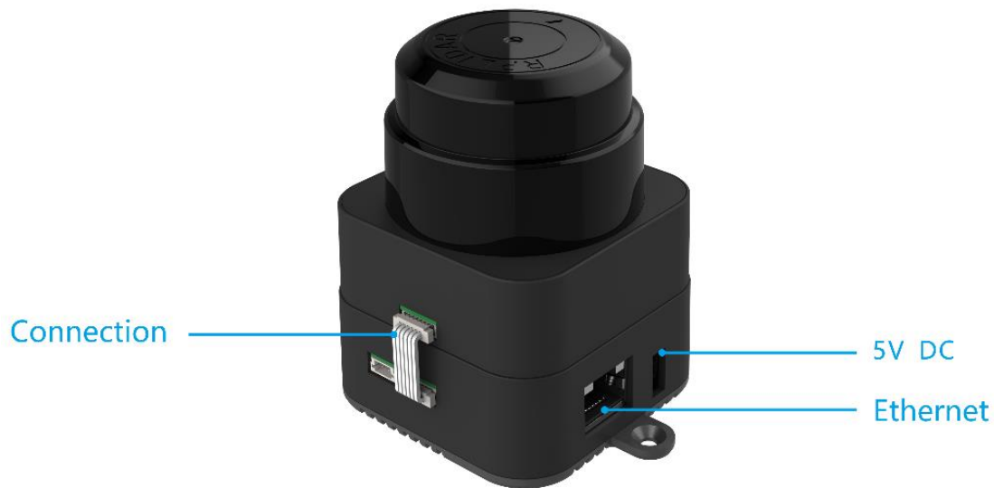
Figure 2-5 SLAMTEC Mapper Professional Kit Interface Definition Diagram
