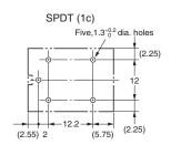
**Terminal Arrangement/** Internal Connections
