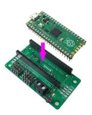
Power is provided via a terminal block connector, the supply is then controlled by an on/off power switch to the board. There is a green power LED to indicate when the board is turned on. The power connections are reverse polarity protected. The board produces a regulated 3V supply that is fed into the 40 way connector to power the Pico, removing the need to power the Pico directly.
