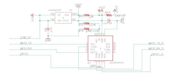
Because this is an analog switch, the nRF52840 current limitations, 2 mA in standard drive (the default), and 9 mA in high drive also apply on the M8 side of the analog switch. The switch is rated up to 300 MHz, higher than the highest UART or I2C baud rate. The 3.3V recommended maximum for GPIO also applies on the M8 connector.
