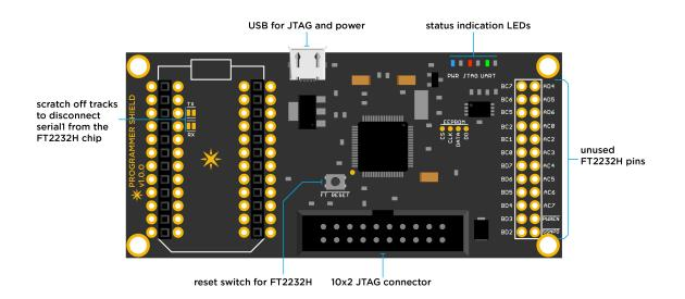
The USB-UART interface is connected to the TX and RX of a Particle device and communicates via Serial1
