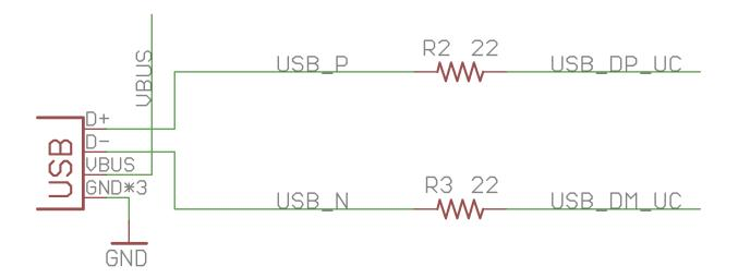
The USB data lines are terminated with 22 Ohm resistors. These data pins are also exposed via small through holes next to the USB connector and are labeled D+ and D-. The VBUS (+5VDC VCC of the USB port) is fed to the PMIC via a 3Amp Schottky diode (SS3P3). The VBUS pin is also available via the unpopulated header hole on the top-right side of the E series.
