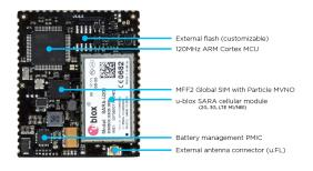
Particle E Series modules 36.0 x 43.0 x 4.6 mm
