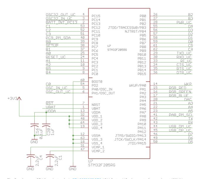
The E series uses ST Microelectronics's STM32F205RGT6 ARM Cortex M3 microcontroller running at 120MHz.
