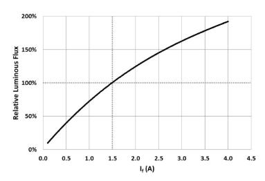
$\varphi_v/\varphi_v$ (1.5A) Single Pulse 20ms  $T_i = 85$ °C
