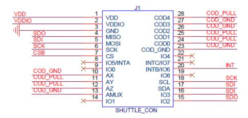
BMP3xy shuttle board electrical layout
