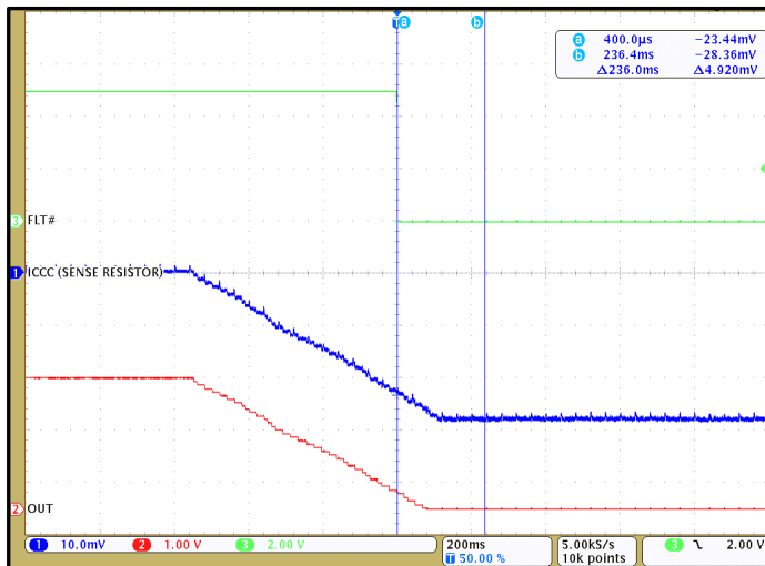
Figure 12. CT428 OCD enabled at -110% of -30 A_{PK} and FLT# is LOW
