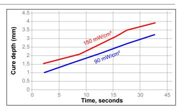
LOCTITE UV8800M can be cured by irradiation with ultraviolet and visible light as well as LED-UV light with single wavelength distribution of sufficient intensity. Cure rate and depth of cure depend on the intensity, spectral distribution of the light source, exposure time and light transmittance of the substrate through which the light must pass.
