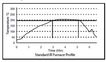
The above cure profile is a guideline recommendation. Cure conditions (time and temperature) may vary based on customers' experience and their application requirements, as well as customer curing equipment, oven loading and actual oven temperatures.
