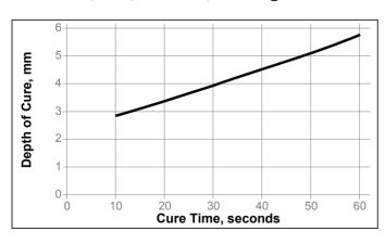
LED Flood Array 405nm, 100 mW/cm<sup>2</sup>, measured @ 405 nm
