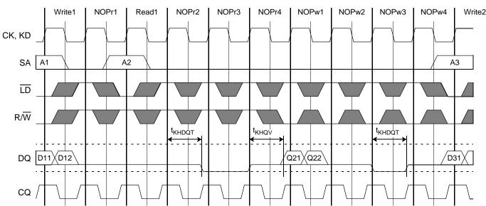
**Note**: In the diagram above, the controller is disabling its DQ ODT except from the beginning of NOPr4 to the beginning of NOPw3. And while it is disabling its DQ ODT, the controller is driving DQ Low when it isn't driving write data. Whereas, the SRAM is enabling its DQ ODT except from the beginning of NOPr2 to the beginning of NOPw3. And while it is disabling its DQ ODT, the SRAM is driving DQ Low when it isn't driving read data.
