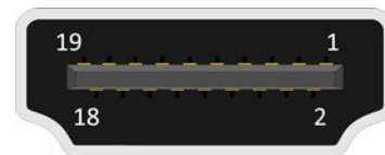
Figure 10: HDMI port diagram
