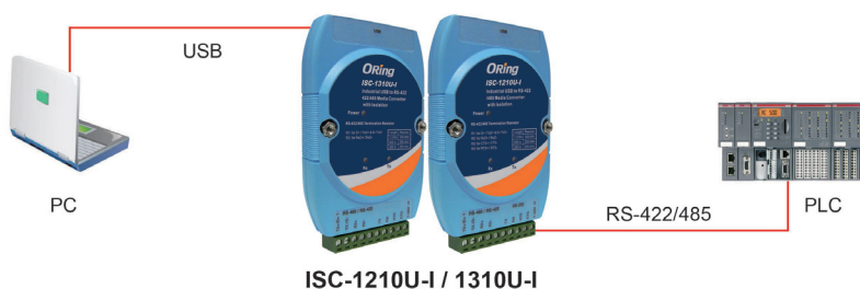
Connections of Media converter
