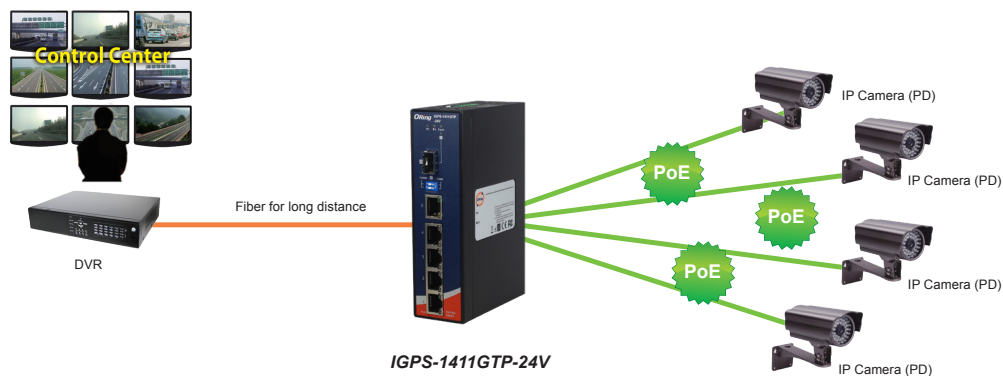
Connections of Ethernet devices
