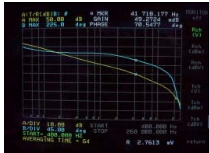
Fig. 6 - Measured loop gain Bode plots.
