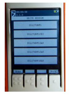
Switch-OFF and ON the Eiger platform to read the new part number from the EEPROM, the firmware will automatically select the right modules settings. Check the Part number of the module plugged on the Eiger platform by clicking on menu ->System->About->Target device.
