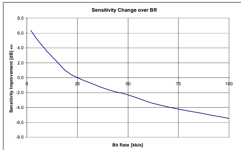
Figure 68: FSK Sensitivity vs. BR
