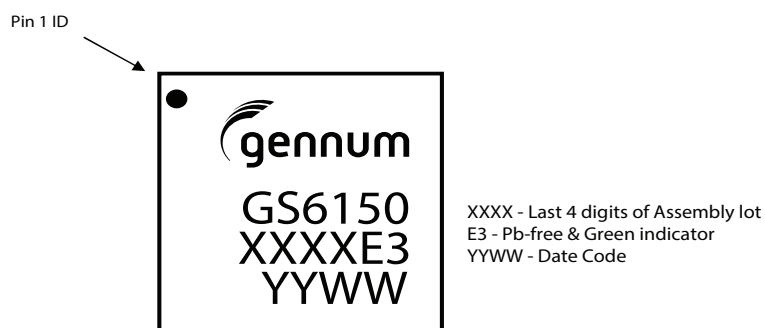
Figure 7-3: GS6150 Marking Diagram
