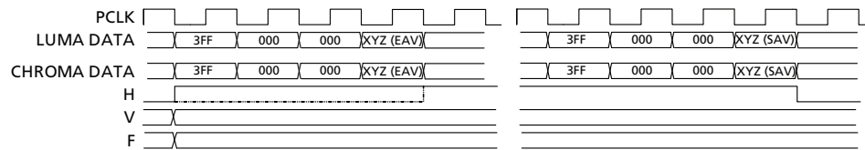
Figure 4-2: H:V:F Output Timing - 3G Level A and HDTV 20-bit Mode
