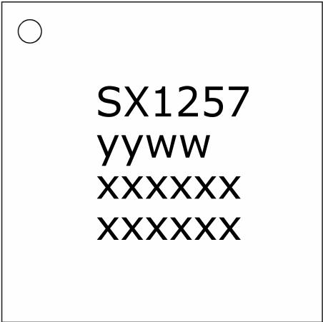
Figure 7-3: SX1257 Marking Diagram
