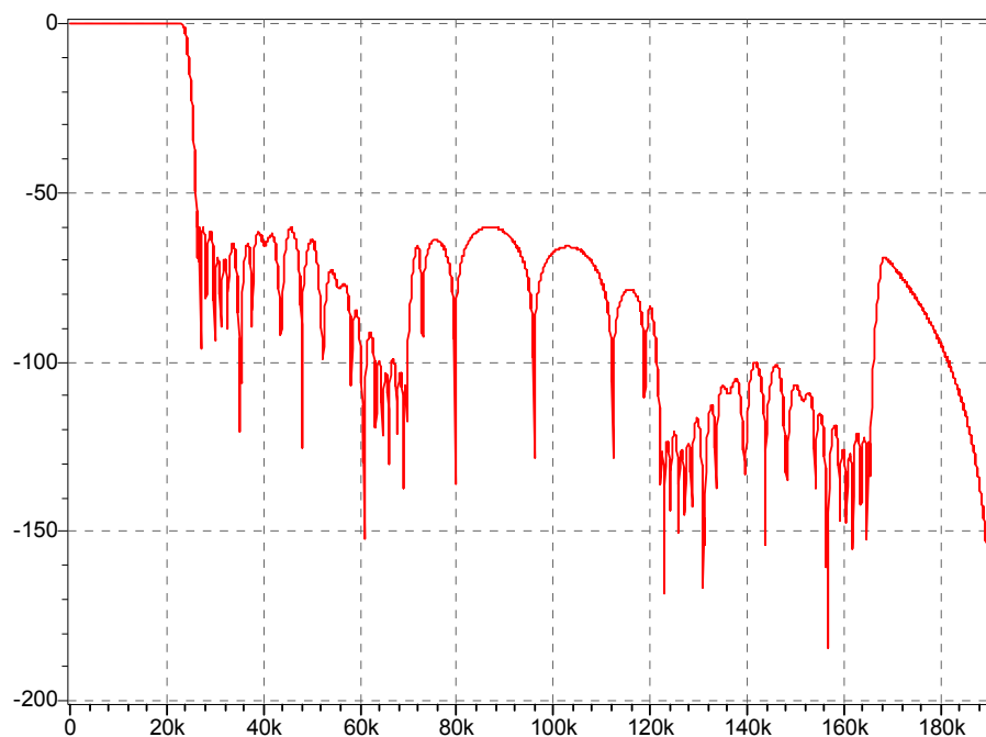
Figure 51 ADC Frequency Response up to 4 \times f_s (Sample rate, f_s = 48\text{kHz} )
