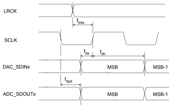
**Figure 6. Serial Audio Interface Master Mode Timing**
