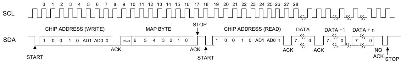
**Figure 24. Control Port Timing, I<sup>2</sup>C Read**
