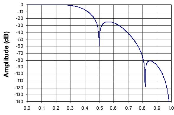
**Figure 39. QSM Stopband Rejection**
