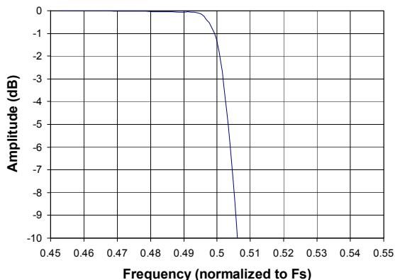
**Figure 33. SSM Transition Band (Detail)**
