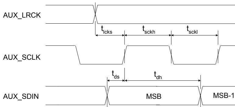
**Figure 7. Serial Audio Interface Slave Mode Timing**
