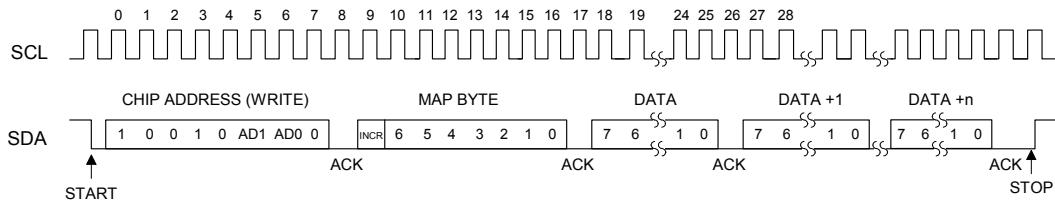
**Figure 23. Control Port Timing, I<sup>2</sup>C Write**
