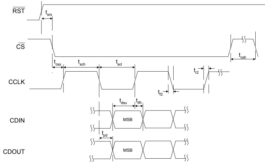
**Figure 9. Control Port Timing - SPI Format**
