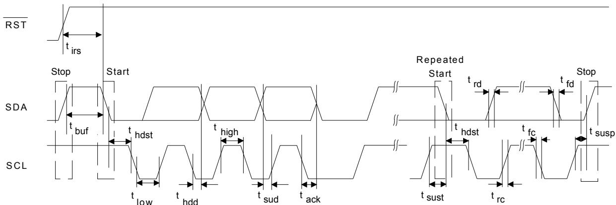
**Figure 8. Control Port Timing - I<sup>2</sup>C Format**
