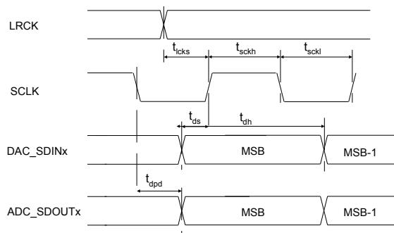
Figure 4. Serial Audio Interface Slave Mode Timing
