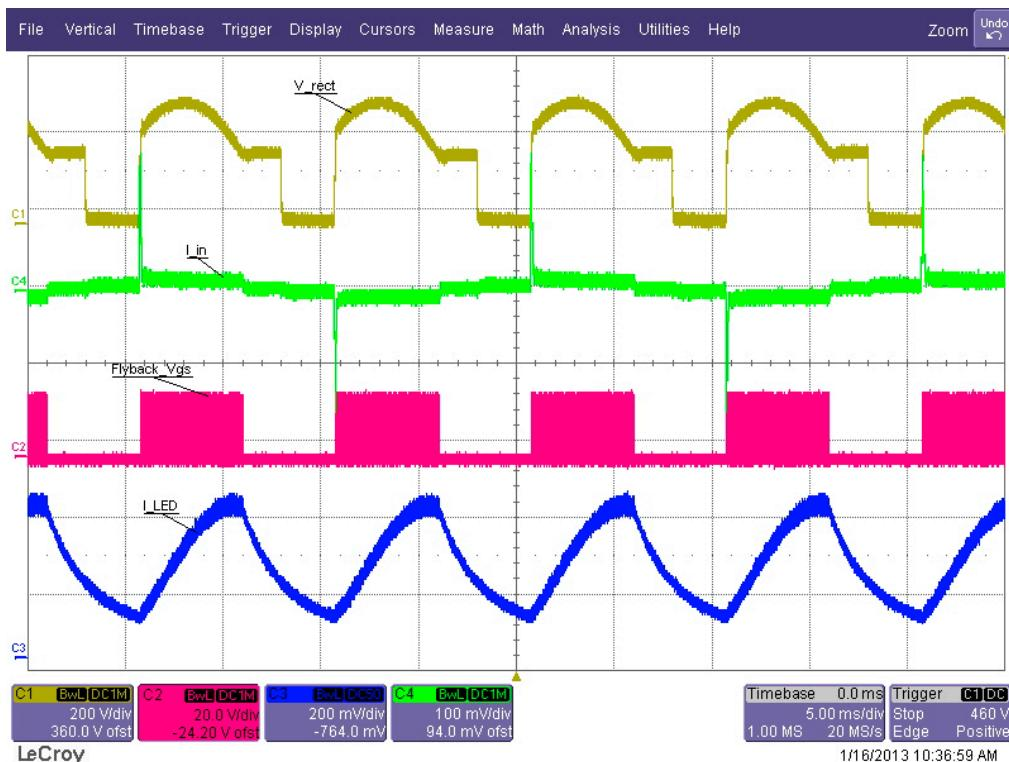
**Figure 21. Leading-edge Dimmer Mode, Steady-state, 230VAC**
