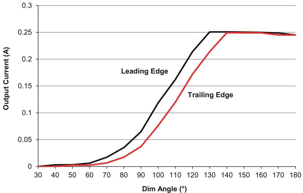
Figure 15. Typical Output Current vs Dim Angle
