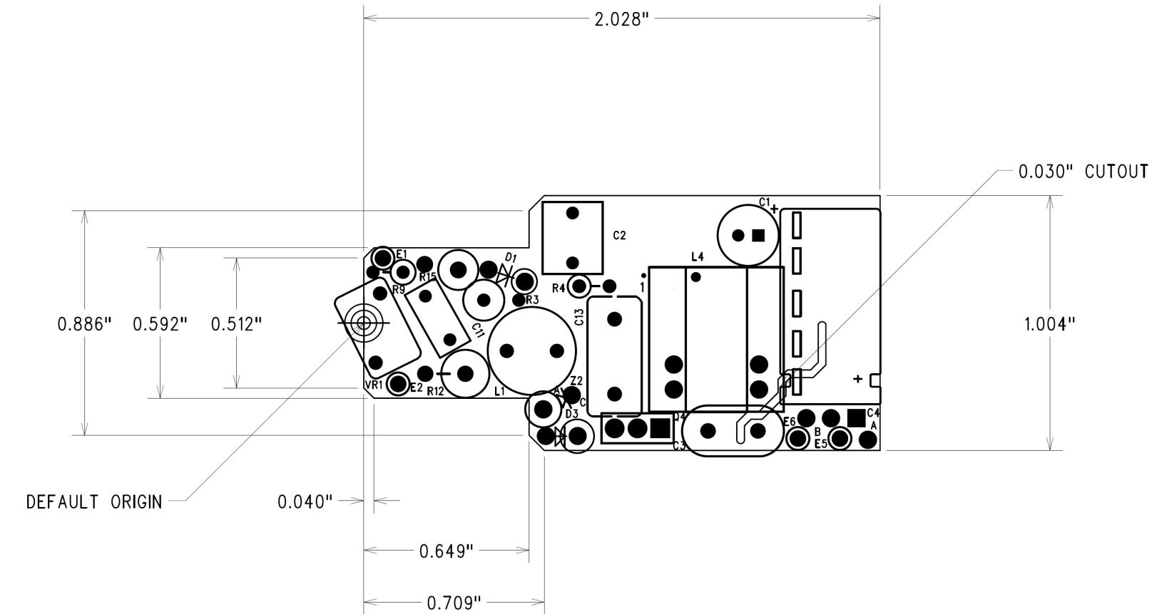
Figure 3. PCB Dimensions
