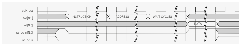
Figure 148. Typical Read Operation in Enhanced SPI Mode
