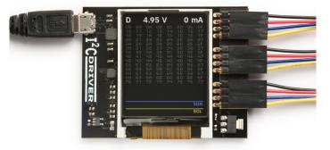
Connect the three sets of colored hookup wires as shown, following the same sequence as on the colored label:
