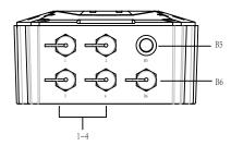
A4 — Antenna interface 1~4 — RS-485 channel interface B5 — Switch/LED indicator light B6 — Power interface
