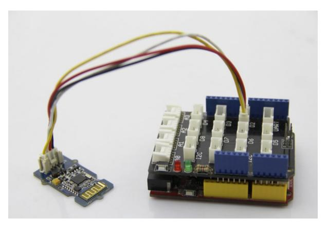
Grove - BLE can be acted as a master or slave, you can use the one via different demos. If you are going to use the following SoftwareSerial program, please refer to the way of connection in the previous pic. TX-->D2, RX-->D3.
