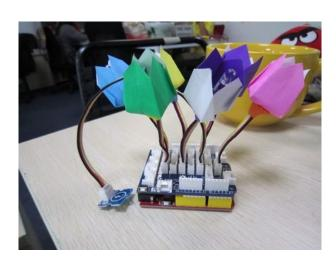
Connect the buds and the touch sensor onto the Grove – Base Shield with the 10cm Grove cable. And then upload the code to your controller.
