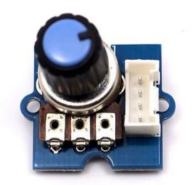
The potentiometer Grove produces analog output between 0 and VCC. The angular range is 300 degrees with a linear change in value. The resistance value is 10k ohms, perfect for Arduino use. This may also be known as a "rotary angle sensor".
