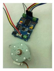
2. Control the Stepper using the I2C motor Driver V1.3 on-chip Atmega8L.
