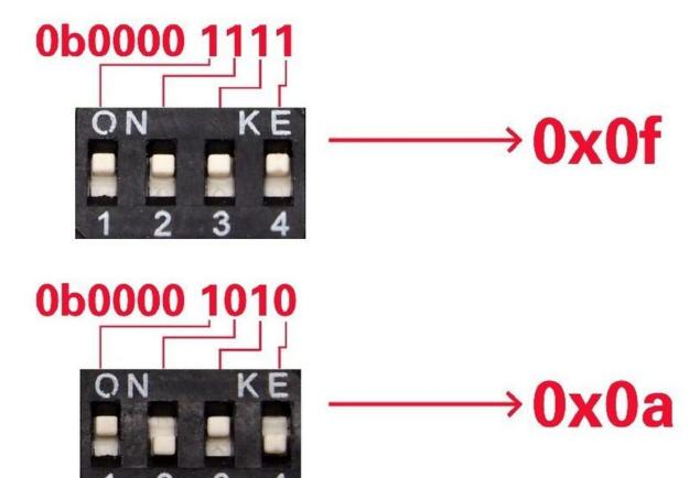
• Then keep the address setup in the program the same as the address setup on the I2C motor driver. The default address setup in the program is 0x0f.
