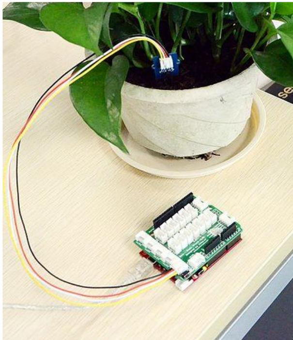
Note: This sensor isn't hardened against contamination or exposure of the control circuitry to water and may be prone to electrolytic corrosion across the probes, so it isn't well suited to being left in place or used outdoors.
