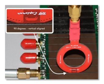
The H-Loop antenna works basically as an inductive coil, capturing magnetic flux.
