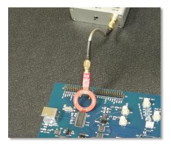
Compared with other near field antennas, RFEAH-25 is smaller and lighter, exactly what fits best when space is constrained in a PCB.
