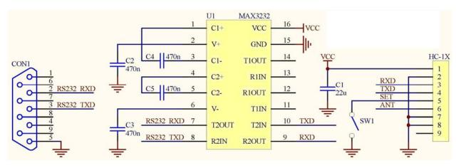
"SET" pin through the switch SW1 grounding can enter the parameter setting state, left hanging out.
