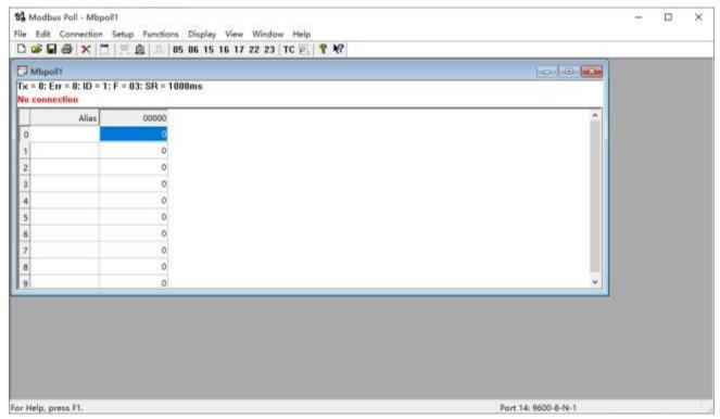
Configure connection parameters: baud rate 9600bps, 1 start bit, 8 data bits, none parity, and 1 stop bit.
