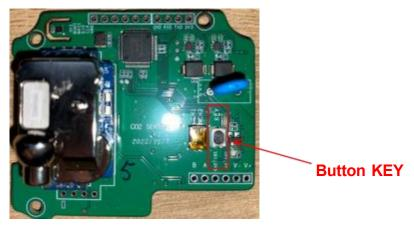
Tips: During the calibration process, the equipment only needs to be powered on all the time without any communication instructions. During the calibration process, the sensor does not respond to any Modbus or SDI-12 requests.
