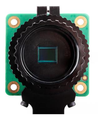
The Raspberry Pi High Quality Camera is the latest camera accessory from Raspberry Pi. It offers higher resolution (12 megapixels, compared to 8 megapixels), and sensitivity (approximately 50% greater area per pixel for improved low-light performance) than the existing Camera Module v2, and is designed to work with interchangeable lenses in both C- and CS-mount form factors. Other lens form factors can be accommodated using third-party lens adapters.
