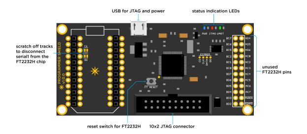
The USB-UART interface is connected to the TX and RX of a Particle device and communicates via Serial1
