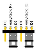
**Software Serial:** Connects easyRadio to Arduino software serial port on D2 and D3
