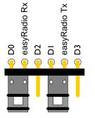
Hardware Serial: Connects easyRadio to Arduino hardware serial port (UART) on D0 and D1
