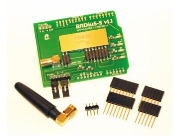
This 'shield' allows Arduino<sup>™</sup> boards to communicate wirelessly using proprietary LPRS 'easyRadio' technology operating in the 433MHz or 868MHz (UK & Europe) & 915MHz (US) Industrial Scientific & Medical (ISM) bands.
