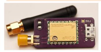
Utilising proprietary LPRS 'easyRadio' technology operating in the 434MHz or 868/915MHz Industrial Scientific & Medical (ISM) bands a pair of eRIC USB 'dongles' can provide a simple 'wireless bridge' between any host devices that support USB serial communications such as a PC or Raspberry Pi <sup>TM</sup> or BeagleBone Black etc.
