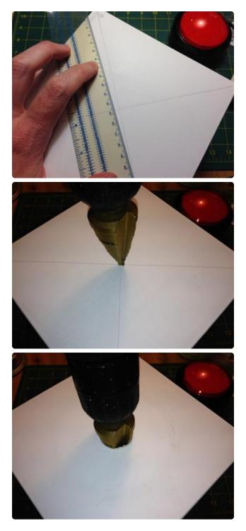
The massive arcade button needs a 1" circular hole cut. Measure to find the center line of your box. Using a step drill bit, drill down until you reach 1".
