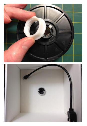
Next, install the massive arcade button on the top of the box. Remove the white plastic locking nut on the bottom of the button. Place the button through the hole and tighten the locking nut from below.
